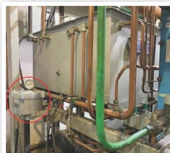
Hydraulic by-pass filter fitment on H.P. Power Pack
