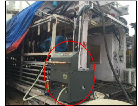
Filtration System attached to a Tunnel Boring Machine
