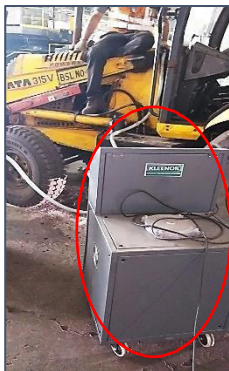
Filtration System attached to a Wheel Loader
