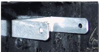
If you cannot accomplish a drill through hole where access will be available for the nuts, you will have to drill and tap the holes using any appropriate bolts you may have. When tightening the tapped bolts, do not over torque. Refer to the chart below when using different bolts for the bracket mount.
