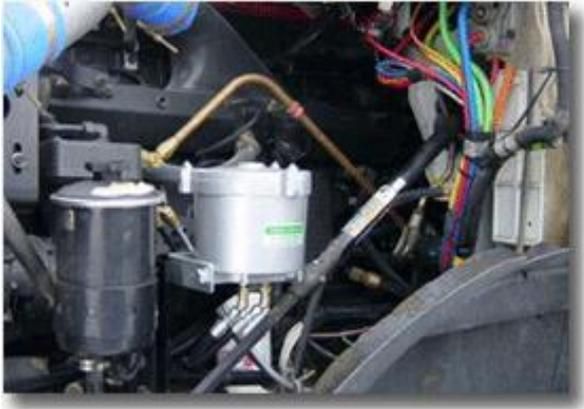
Locate as many drain or return ports as possible. Return ports are generally on the engine block and can be found near the dipstick or in the engine sump pan.
