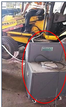
Filtration System attached to a Wheel Loader
